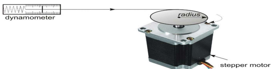
Figure 5. Torque measurements set up..
